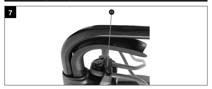
Hook the mains cable through the cable strain-release 11 to reduce the strain on the cable fitting as you mow.
