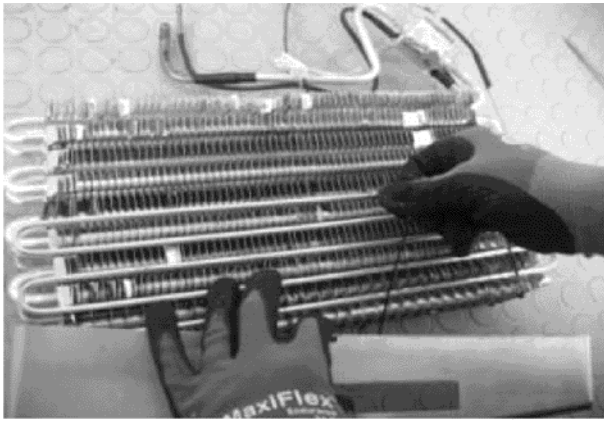
10. Tie the tray and thermal fuse to the evaporator with cable tie.
