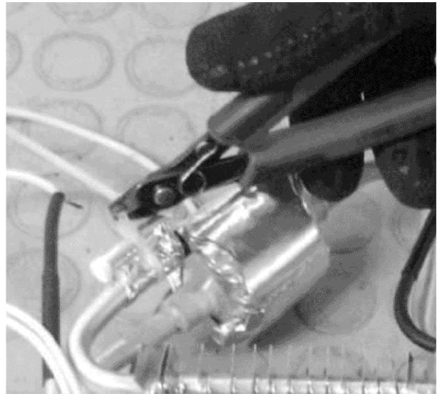
12. Place the new Evaporator Assy. to its place, when fixing the Evaporator Assy. press it horizontally otherwise you might damage the fixing plastics.
