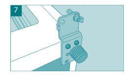
Tilt the fridge freezer back, no more than 45°, to access the bottom hinge and feet. Remove the feet and the bolts securing the right hand hinge plate and the left hand fixing plate.
