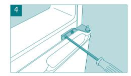
Remove the middle hinge using the 8mm socket or spanner. Take care not to lose the spacer if fitted. Lift the freezer door off the bottom hinge.
