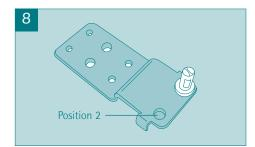
Remove the hinge pin from position 1 and replace it in position 2. Place the hinge on the opposite side of the cabinet, secure it with the three bolts, and screw in the foot into position.
