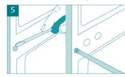
Remove the blanking plates and screw cover. Remove screw and replace screw on the opposite side.
