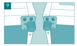
Place the fixing plate on the opposite side of the appliance, secure it with the three bolts, and screw the foot into position.
