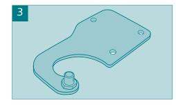
Remove the pin from the bracket and replace it into the same hole from the other side.
