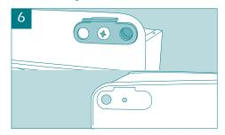
Remove the hinge insert plate from the bottom of the fridge and freezer doors. Replace the plate on the opposite side.
