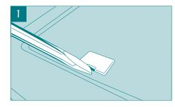
Remove the four blanking plates from the top of the fridge freezer with a flat bladed screwdriver. Remove the screws underneath with a Phillips screwdriver.
