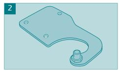
Use the 8mm socket or spanner to remove the three bolts above the door hinge. Lift off the bracket. Remove the fridge door.
